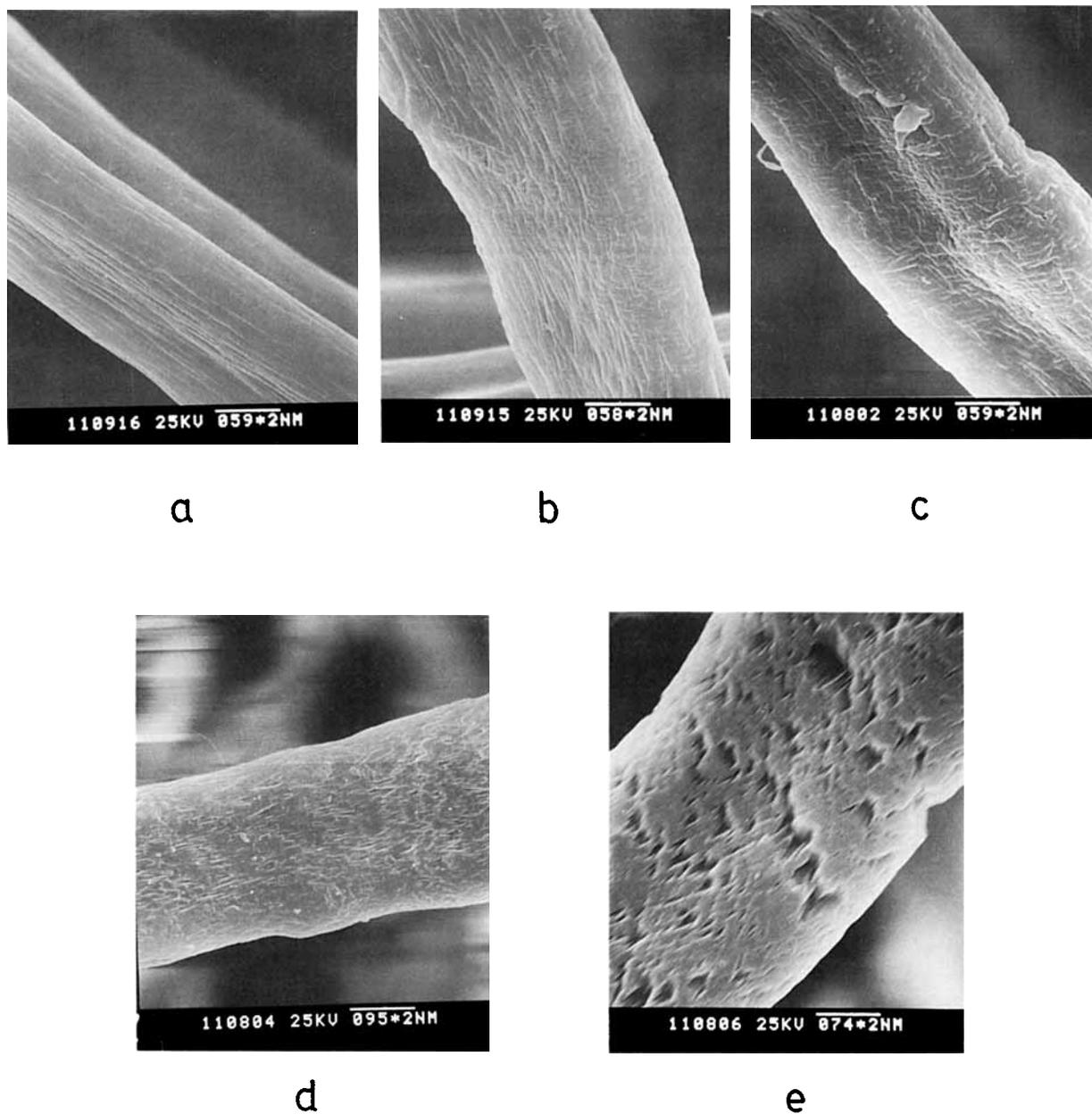
**Figure 6** Scanning electron microscope photographs of the fibers amidoximated at various temperatures: (a) before reaction; (b)  $65^\circ\text{C}$ ; (c)  $70^\circ\text{C}$ ; (d)  $75^\circ\text{C}$ ; (e)  $80^\circ\text{C}$ .
