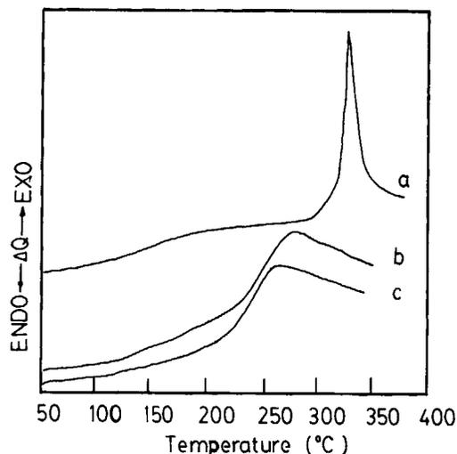
**Figure 10** DSC curves of the fibers with various nitrile group conversions: (a) 0%; (b) 5.4%; (c) 28.4%.
