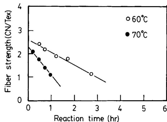
**Figure 8** Effect of reaction time on the strength of fiber: concentration: 100 g/L.
