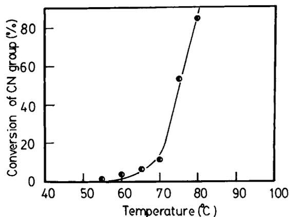
**Figure 7** Effect of temperature on nitrile group conversion: time, 30 min; concentration, 100 g/L.
