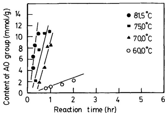
**Figure 4** Effect of reaction time on the content of amidoxime group at various temperatures; concentration: 100 g/L.
