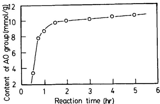
**Figure 3** Effect of reaction time on the content of amidoxime group: temperature, 80°C; concentration, 100 g/L.
