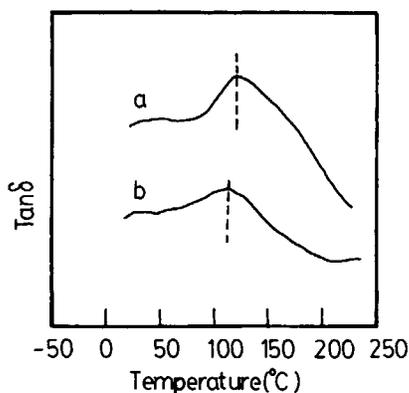
**Figure 9** Temperature vs. loss tangent: (a) PAN fiber; (b) amidoximated PAN fiber with nitrile group conversion of 28.4%.
