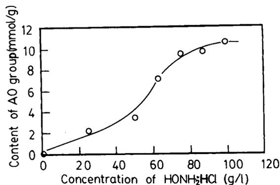
**Figure 2** Effect of hydroxylamine hydrochloride concentration on the content of amidoxime group: temperature, 80°C; time, 30 min.
