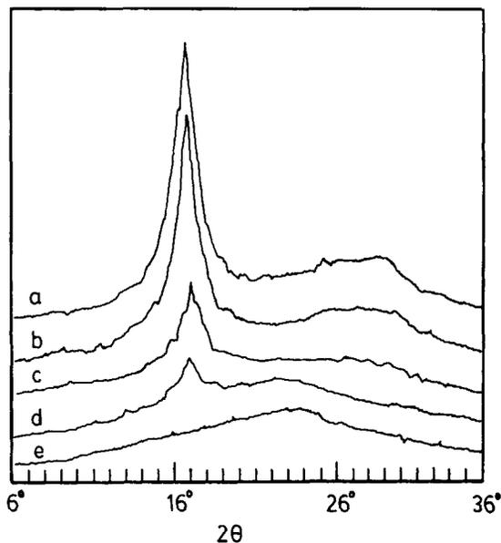
**Figure 5** WAXD diagrams of the fibers amidoximated at various temperatures: (a) before reaction; (b) 65°C; (c) 70°C; (d) 75°C; (e) 80°C.
