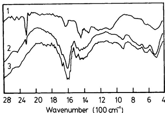
**Figure 1** IR spectra of fibers with various nitrile group conversions: (1) 0%; (2) 53.7%; (3) 98.4%.
